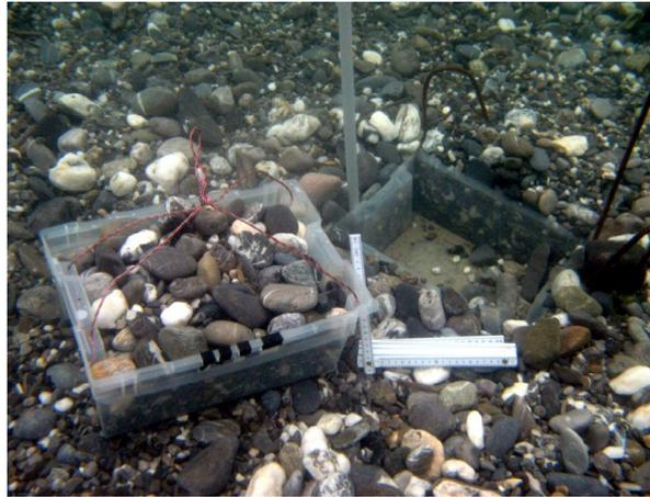
FIGURE 3 Experimental container on the top of the fill in the site Litzelstetten-Krähenhorn (KRAH), November 2009, before inserting it into a nestable container of the same size (behind right). The container had been filled with the same bulk material and served for invertebrate sampling and for colmatation experiments.
